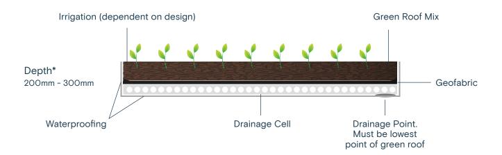
\*Know the weight the roof/slab can hold to calculate the kg/m². The depth of media can be calculated using Saturated Bulk Density value. Optimum depth is 300mm.
