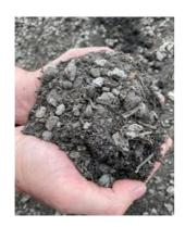
The B Horizon Mix performs well as a lower profile substrate in contained environments, below the Lightweight Planter Box Mix. It has been developed to work as the stable drainage media layer of an engineered profile. It provides enough nutrition for continued root growth while creating a stable substrate for long term volume.
